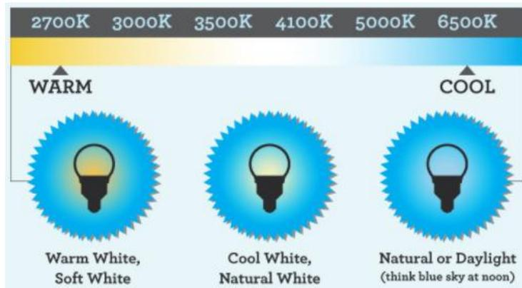
Figure 4. Color temperature of LED lamps
